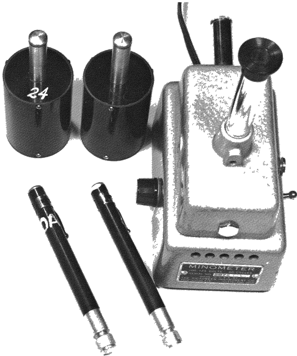
Fig. A.9—Ionization chambers and charger-reader.
